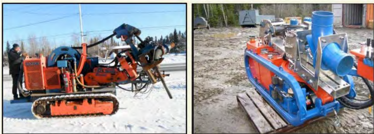
Fig. 14 (above) -- The Company has two models. The normal Dragon unit (seen left, above) is on tracks, it can also accommodate a drill. The Mini-Dragon unit (seen right, above) is very small, it will fit in small drifts. Nippon Resources Inc. has a manufacturing hub in the Val d'Or area of northern Quebec. Right now it is in a position to produce 2 to 3 Dragon units per month. The unit is designed for toughness, and parts for the Dragons can be replaced using standard Caterpillar-type parts, apart from the burner head (which comes from the Company). Under normal use the burner head typically has a lifespan of ~1yr before pro-active replacement.
