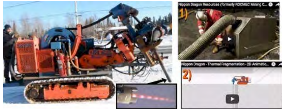
Fig 1. (above - left) Thermal Fragmentation Dragon unit with inset of burner. (above - right) Click to view videos; 1) in operation, & 2) 2D animation of uses.
