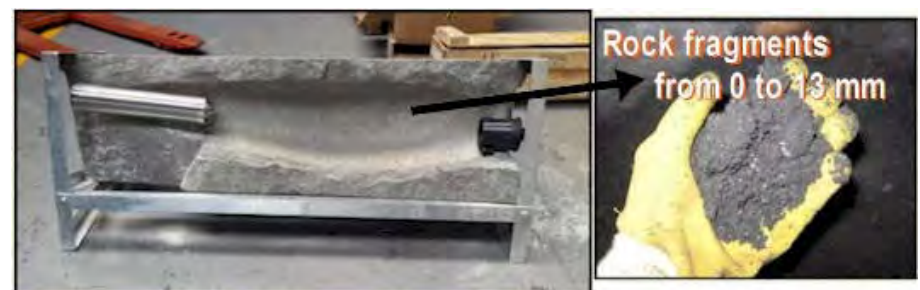
Fig 2. (above) Thermal Fragmentation technology is precise and surgical, extracting only the vein with minimal dilution. Above is seen a cross section of thermally fragmented rock, and sample of fragmented mineralized ore (rocks ranging from 0 to 13 mm in size). Typically the hardest rock will fragment first -- precious metals are found in quartz vein, which is harder than surrounding waste. When the process is started it makes an oval hole and essentially searches the quartz before the waste -- the operator can both see and hear when quartz is being extracted vs. waste.
