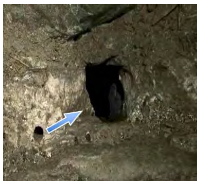
Fig. 10 (above left) -- Precision thermal fragmentation minimizes dilution.
