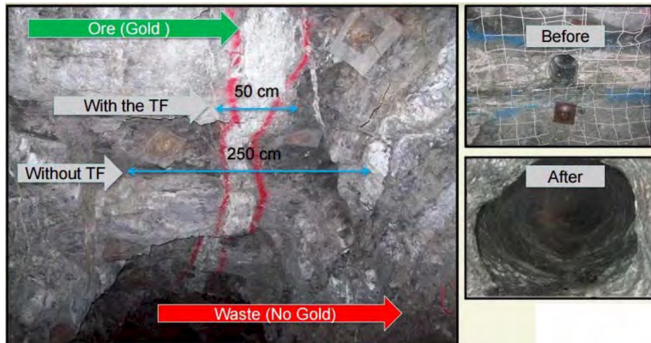
Fig. 9 (above left) -- Image of vein annotated with the degree of accuracy that thermal fragmentation works relative to without, (above right) from pilot hole to ~1 x 1 m.
