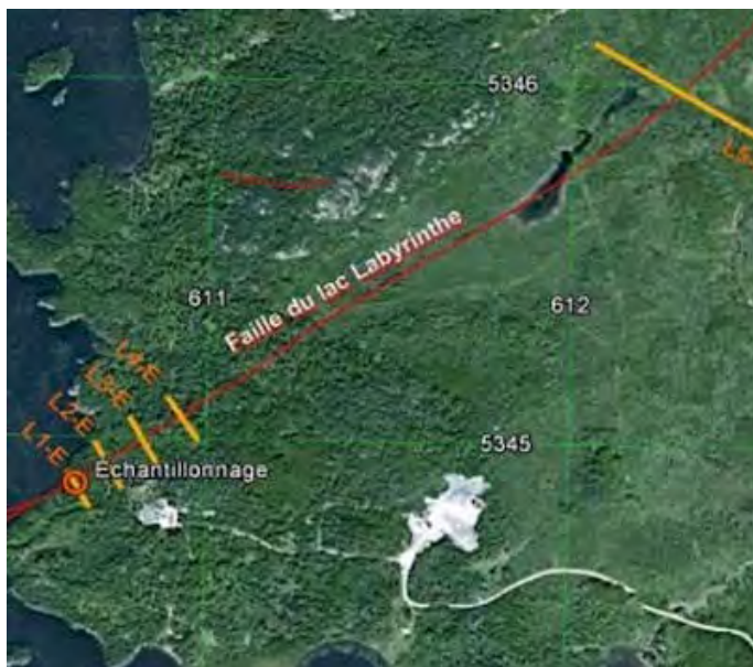
Fig. 18 (above) -- Mineralized Boucher structure/veins coincides with the Lac Labyrinthe Fault (annotated on satellite view of area). The width of the structure is ~30 m, and it runs for >3.5 km on the property.
