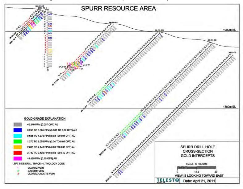
Figure 19.17: Drill Hole Gold Intercept Cross-Section – Spurr Resource
