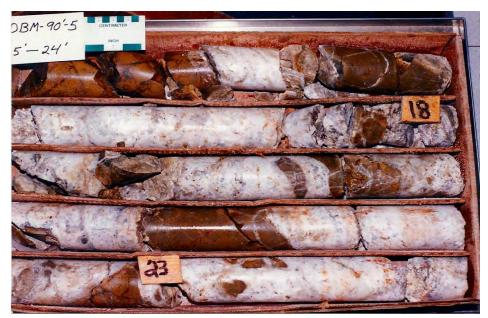
Figure 13.3: Core From Degerstrom Hole 90-5 (14.5–24 ft)
