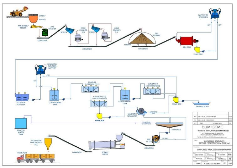
Figure 17-1: Process Flow Diagram
