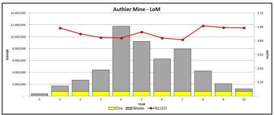
Figure 16-9: Mill Feed Grade (Li<sub>2</sub>O), Resources and Waste Production
