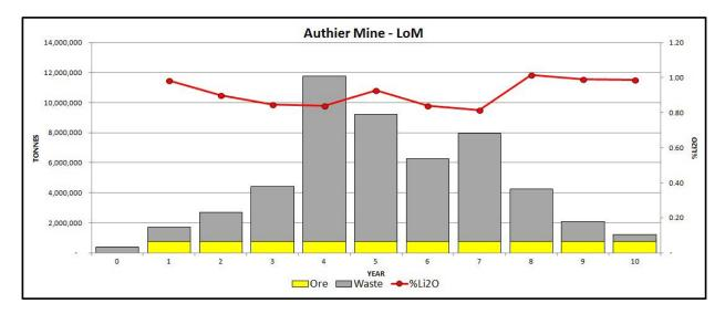
The production was planned over 350 days per year, on two 10 hour shifts per day. The main mining fleet will consists of hydraulic excavators of 6 m<sup>3</sup> bucket capacity, and 37 tonnes off-road trucks. The following Table is listing the main open-pit equipments.
