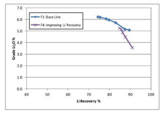
Figure 8: Spodumene Flotation Plots from Test F1 and F4
