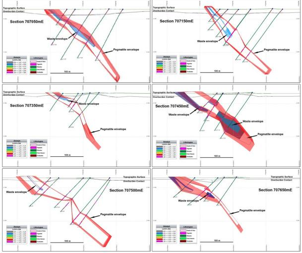
Figure 14-4: Modeled Envelops with Mineralised Intercepts on Sections (looking west)
