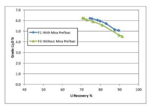
Figure 7: Effect of Mica Pre-Float on Spodumene Flotation
