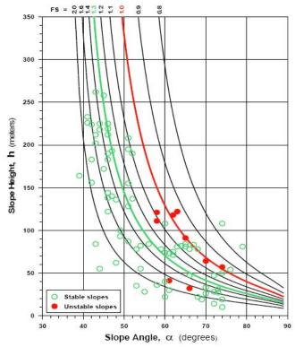
Figure 16-1: Cases of Rock Slope With Stable and Failed Conditions Distinguished<sup>1</sup>
