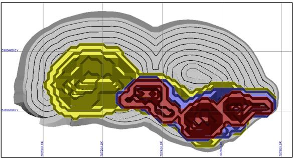
Figure 16-8: Plan View of the Optimal Open-Pit
