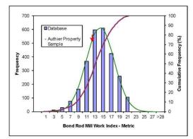
Figure 3: Head Composite Bond Rod Mill Work Index Comparison to SGS Database
