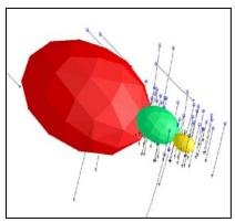
Figure 14-7: Search Ellipsoids used for the Interpolation Process
