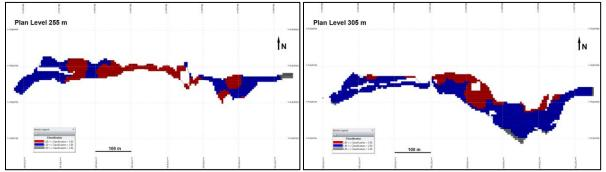
Figure 14-11: Level Plan Views Showing Li<sub>2</sub>O Block Model Interpolation Results
