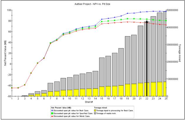
Figure 16-2: Pit Tonnage versus NPV (\$) showing Optimal Shell
