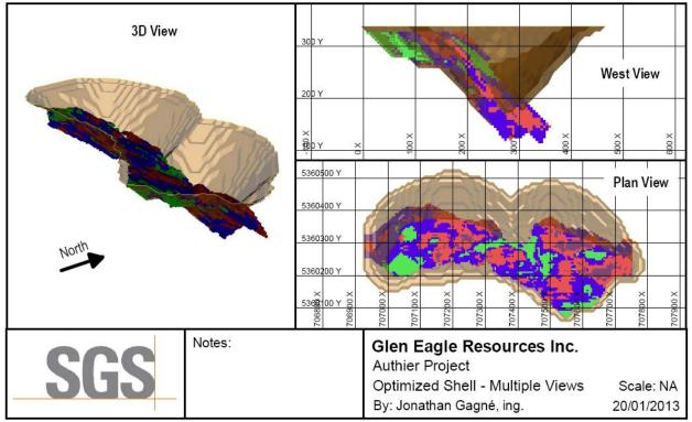
Figure 16-3: Multiple Views of the Optimized Shell
