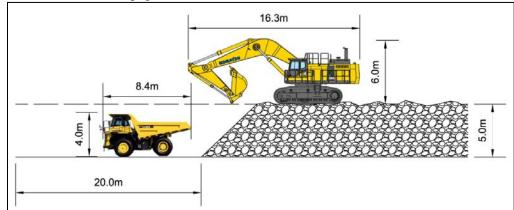
Figure 16-6: Minimum Push-back Width
