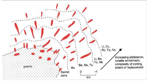
Image from Sinclair 1996 (modified from Trueman and Cerny 1982) Figure 8-1: Schematic Representation of Regional Zonation of Pegmatites
