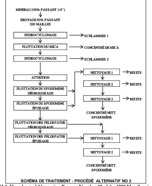
Figure 13-1: Flowsheet of Alternative Process Number 12 of the 1999 Metallurgical Study
