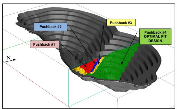
Figure 16-7: Typical Section View of Pushback's 1, 2, 3 and 4 (Optimal Pit Design)
