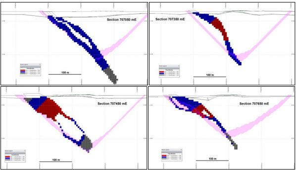
Figure 14-10: Sections Showing Li<sub>2</sub>O Block Model Interpolation Results
