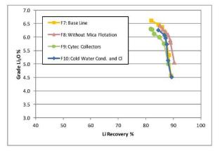
**Figure 10: Final Development Flotation Test Results**
