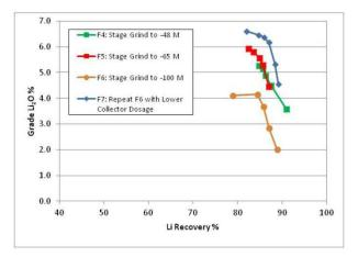
Figure 9: Effect of Grinding Fineness on the Spodumene Flotation Performance
