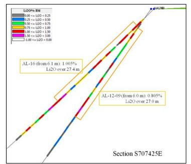
Figure 12-2: Oblique View Showing Results for Twin Holes Al-16 and AL-12-09
