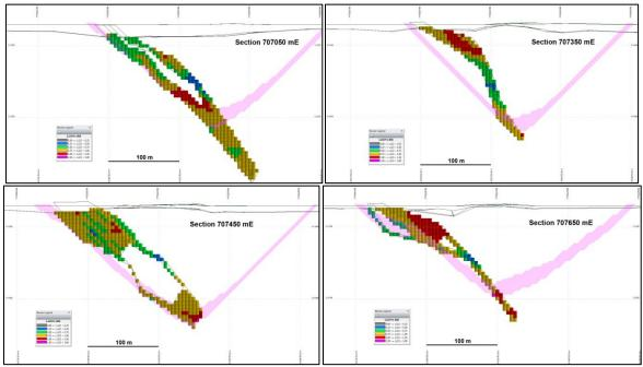
Figure 14-8: Sections Showing Li<sub>2</sub>O Block Model Interpolation Results
