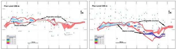
Figure 14-5: Modeled Envelops with Mineralised Intercepts on Level Plan Views
