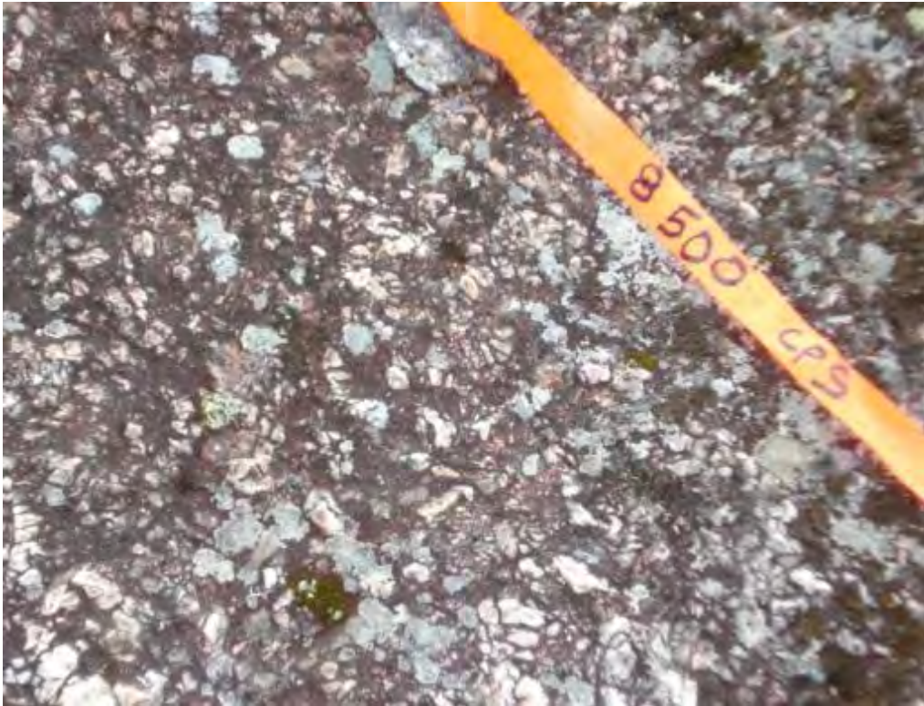
Figure 8.4: Cataclastic H. Peg (w) with hematized matrix, channel MB-01
