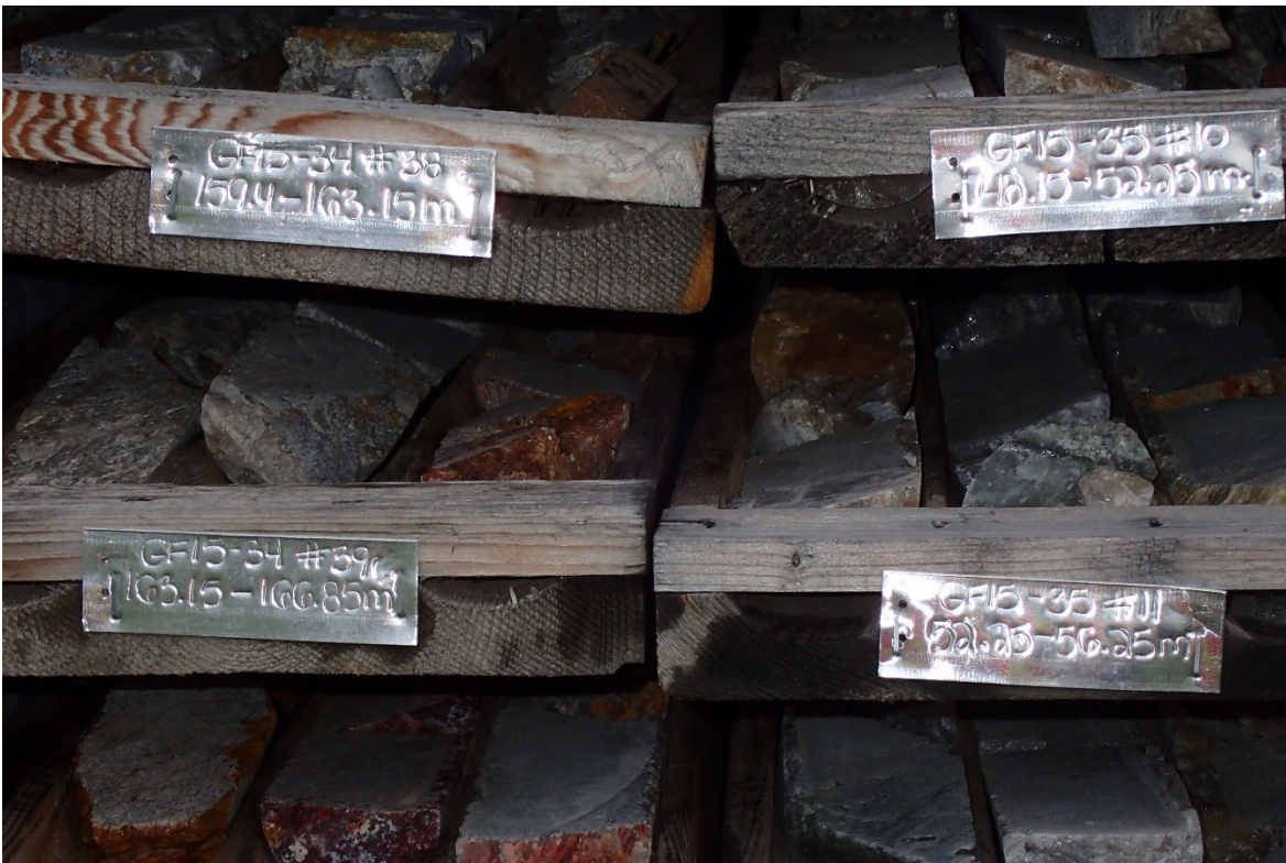
Photo 12: Core Boxes at Core shed with Identification
