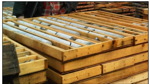
Figure 11-4 - Azure Core in Rehabilitated Boxes (Dec. 7, 2010)
